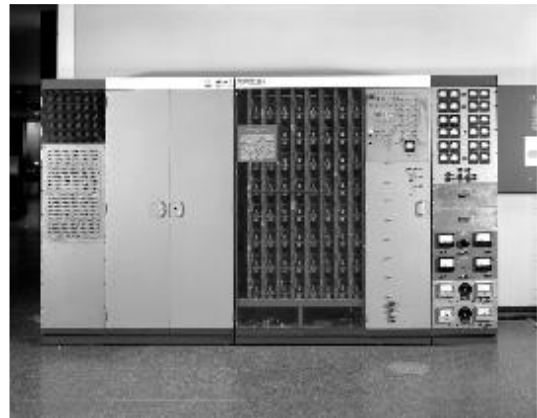
Figure 1. This machine, called the Mark 1 Perceptron, was used to model a single neuron in the 1950s. It had a camera attached to it and was trained to classify pictures of men and women.
