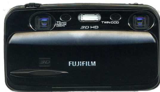
Figure 1. Stereo 3-D camera by Fujifilm. Note that there is a pair of camera lenses at the top – each lens with its own image sensor.
